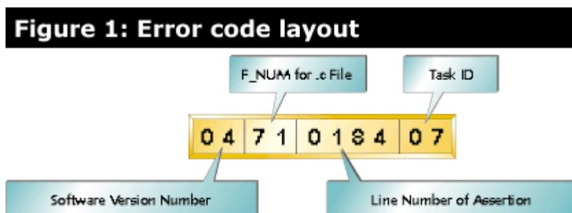
It is also useful to report the number of the task that was running when **aFailed()** was called. This leads to an error code with the layout shown in Figure 1. The user need not be aware of the meaning of each part of the number, but it can be deciphered once the report reaches the engineer who is troubleshooting the failure.
