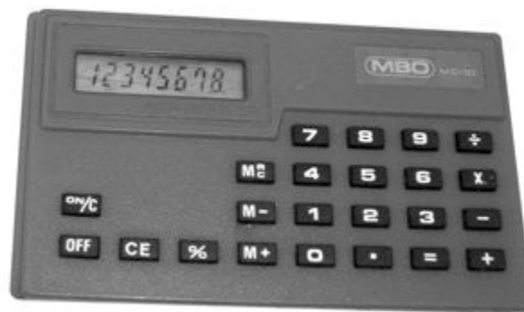
Figure 3-13: A simple electronic calculator used as a model for the statechart example.
